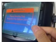
2) The lens cover will loosen and allow you to remove it.
